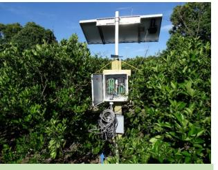
Use of sapflow sensors supported by a datalogger, solar panel, and 12-V battery (right and top)
