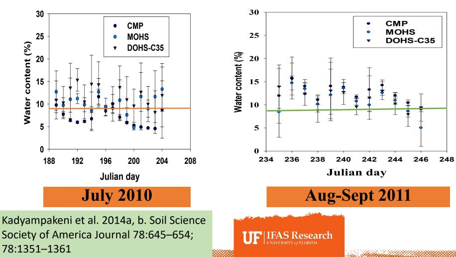
CMP-Conventional microsprinkler irrigation MOHS-Microprinkler open hydroponic system with daily irrigation and weekly fertigaton. DOHS-C35-Drip open hydroponic system with daily irrigation and fertigation
