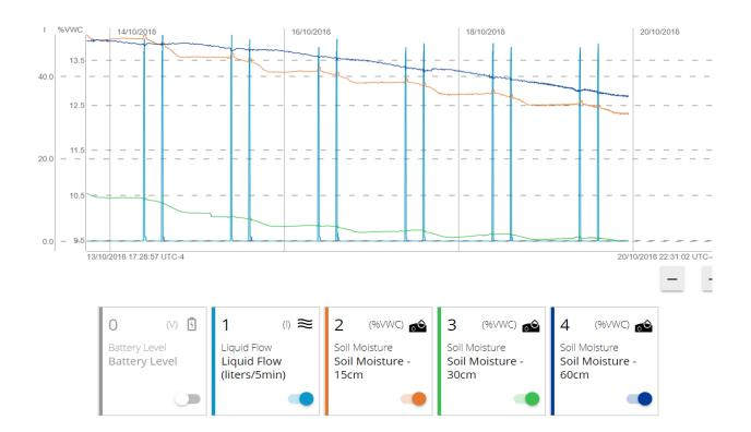
Water monitoring at grove scale and soil moisture distribution at 15, 30 and 60 cm soil depth
