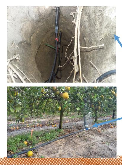
Water monitoring at grove scale and soil moisture measurement at 15, 30 and 60 cm soil depth
